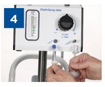
Attach the spray set to the DUPLOSPRAY. Connect the clear hooded luer connector on the tubing set to the male clear gas port on the regulator. Connect the blue male luer connector on the tubing set to the female luer blue vent port on the regulator.
