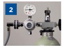
Attach the supply hose located at the back of the regulator to a source of medical grade CO<sub>2</sub>.
